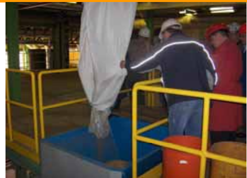
Sand being dumped into hopper
