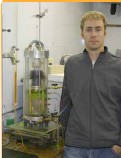
Bryan Bale with one-dimensional freezing cell used to measure effects of freezing and thawing of mine tailings.
