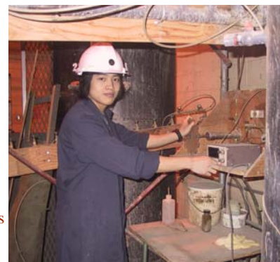
Silawat Jeevaripoolvam, M.Sc. Student, evaluates Creep Compression of Mature Fine Tailings in 10 m high columns. (See page 3.)
