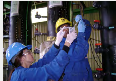
Carmen Li and Saidul Alam (PhD, Geoenvironmental Engineering) collecting a sample from the large settling columns.
